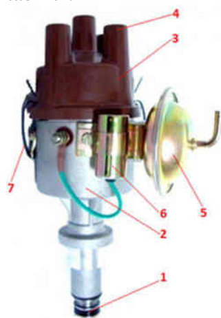
Fig. 2.60 – Ruptor-distribuitor: 1 – arbore de antrenare; 2 – corp; 3 – capac distribuitor; 4 – borne laterale; 5 – regulator de avans vacuumatic; 6 – condensator; 7 – cleme de fixare
